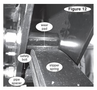
bolt hole, the wear pad, and then out the other side. Finish with a 9/16" nylock nut. Note: When positioned correctly, the wear pad will be above the end of the leaf spring. The spring will contact the wear pad once the suspension is loaded (Figure 12).
