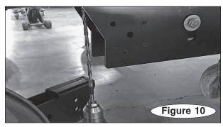
**10.** Use four of the included 3/8" self-tapping screws to attach the slipper spring box to the frame using the holes you just drilled. Use threadlocker on the screws; tighten to 40 lb-ft.
