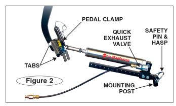
If the cylinder is not pulled back when it is connected, the weight of the cylinder will cause the pedal clamp to depress the towed vehicle's brakes continuously.
