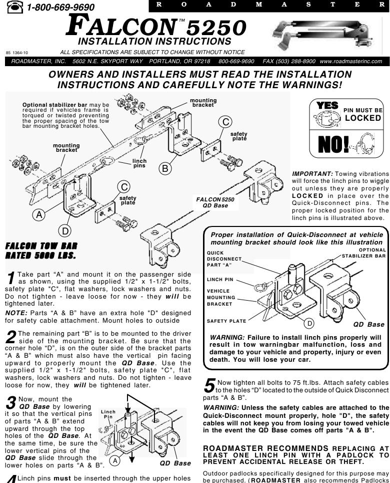
**4** in parts "A & B" and **locked** as illustrated in the column above to keep the **QD Base** stabilized.
