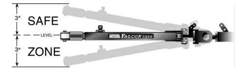
Towing with an upward or downward slope of the tow bar puts undue strain on the tow bar and mounting brackets. **DO NOT TOW if the FALCON is over 3 inches off level as shown** (see CAUTION below). To determine if your bar is at a safe angle:
