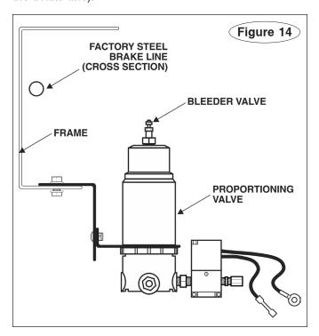
**E.** The closer the proportioning valve is to the air compressor, the less air line will have to be routed between them later.
