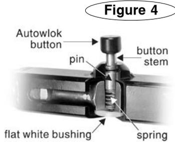
Then, slide the inner arm into the outer arm until the top of the button stem is visible through the hole in the outer arm.
