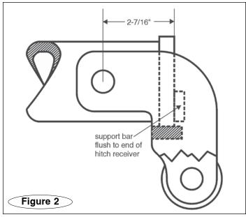
2. IMPORTANT - check the fit. The Rollaway is designed for a standard hitch receiver with a distance of 2-7/16" between the center of the hitch pin hole and the end of the hitch receiver, as shown in Figure 2.
