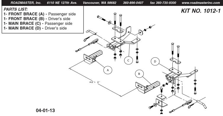
**IMPORTANT:** All baseplates **must** be assembled with all the bolts left loose for final adjustment and positioning (before tightening) unless otherwise instructed. All bolts **must** be torqued for proper strength. If more than one bolt is used per fastening point, the diagram may only show one.
