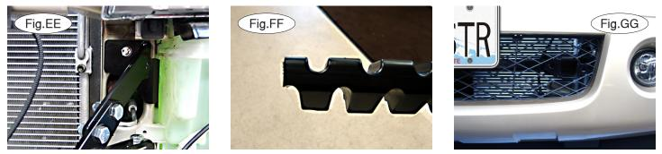
27. Insert the  $\frac{1}{4}$  x  $\frac{1}{2}$  nutted backing plate through the engine compartment. Place the backing plate against the rear frame rail. Bolt into place using a  $\frac{3}{8}$  x  $\frac{1}{4}$  bolt and lock washer (Fig.EE). Repeat for the other side.
