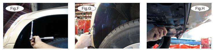
4. Remove one 10mm (head) screw attaching the corner of the fascia to the fender (Fig.F). Repeat for the other side.
