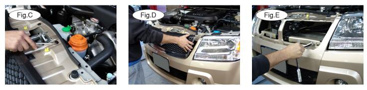
1. *Important:* please use all supplied bolts and parts and read all instructions carefully before beginning this installation. The majority of questions you may have can be answered within the text, and proper installation will ensure safe and secure travel. Now, begin the installation by removing eight plastic fasteners that hold the top of the fascia to the core support (Fig.C).
