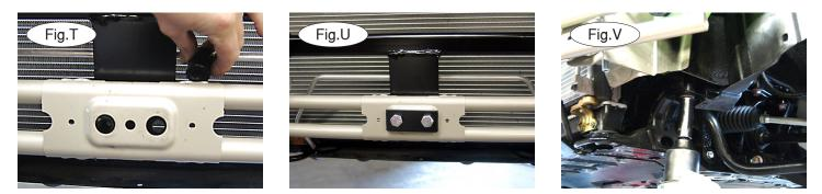
16. Next, insert two 1" x 1<sup>1</sup>/<sub>4</sub>" pipe spacers in the center of the bumper core (Fig.T). The spacers should align with the existing holes in the bumper core and the main brace.
