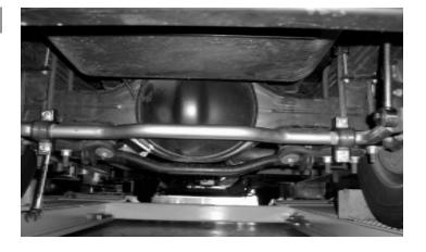
\*Before you begin, inspect the vehicle's U-bolts that will be reused in the installation of this kit. Consider replacing them if they are rusty or show other signs of structural wear.\*
