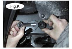
6. Replace the frame caps you removed in step 2, and bolt through the lower part of each main brace with a 12mm x 1.25" x 40mm bolt, flat washer and lock washer (Fig.I).
