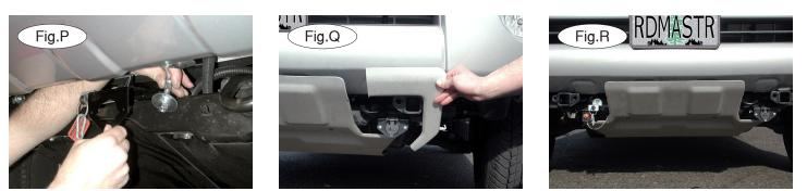
10. Bolt the supplied light plug bracket to the frame cross member, using one of the pre-existing holes. Use a 1-3/8" x 2" bolt, fender washer, lock washer and nut (Fig.P).
