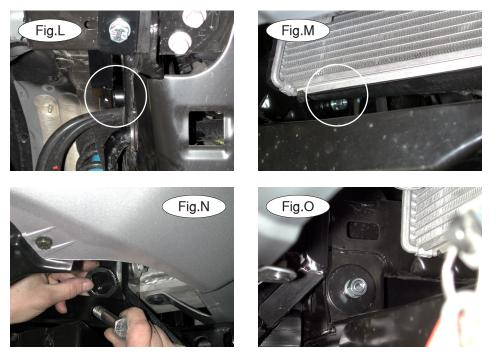
outside of the frame, bolt through the existing hole with a  $\frac{1}{2}$ " x 4" bolt (Fig.M). From the inside of the frame, thread a  $\frac{1}{2}$ " plate washer, lock washer and nut onto the bolt to secure it (Fig.O). Repeat for the other side.
