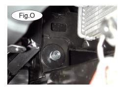
side of the frame, bolt through the existing hole with a ½" x 4" bolt (Fig.M). From the inside of the frame, thread a ½" plate washer, lock washer and nut onto the bolt to secure it (Fig.O). Repeat for the other side.
