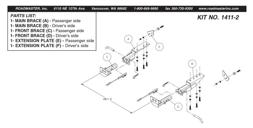
**IMPORTANT:** All baseplates **must** be assembled with all the bolts left loose for final adjustment and positioning (before tightening) unless otherwise instructed. All bolts **must** be torqued for proper strength. If more than one bolt is used per fastening point, the diagram may only show one. Use flat washers over all slotted holes and lock washers on all fasteners.
