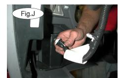
7. Pull down and away on each side of the front fascia (Fig.H), and remove the marker lights (Fig.I) and the turn signal plugs (Fig.J). Remove the fascia.
