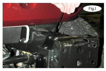
5. Working on the driver's side, place the main receiver brace over the end of the frame rail (Fig.H). Place one of the supplied 3/16" x 1½" x 3½" threaded backing plates with wire through the opening to the inside edge of the frame rail (Fig.I). Using the two supplied ½" x 1¼" bolts and lock washers, bolt through the driver's side main receiver brace, frame rail and into the threaded backing plate with wire (Fig.J).
