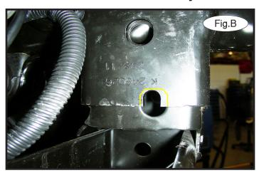
1. Remove the front 10mm nut (Fig.A) and pull the pump off to the side. Then, using a die grinder, enlarge the lower slot in the pump mounting bracket to match the size of the innermost hole (Fig.B). The yellow lines show the approximate area that needs to be enlarged.
