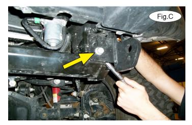
4. Fit the main receiver brace around the lower subframe, aligning the lower holes with the pre-existing holes in the subframe. Use a support stand, if necessary.
