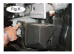
5. Remove the large black air box on the driver's side (two 10mm head bolts – Fig.K). *Note:* on some late model cars, you may not be able to remove the air box. If this is the case, remove the bolts and move the air box off to the side (Fig.L) to allow sufficient working room.
