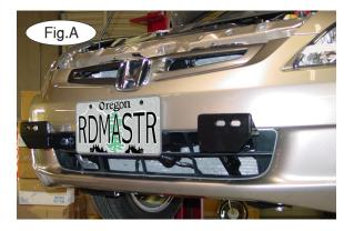
**IMPORTANT:** All baseplates **must** be assembled with all the bolts left loose for final adjustment and positioning (before tightening) unless otherwise instructed. All bolts **must** be torqued for proper strength. If more than one bolt is used per fastening point, the diagram may only show one. Use flat washers over all slotted holes and lock washers on all fasteners.
