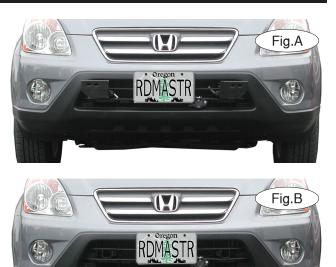
**IMPORTANT:** All baseplates **must** be assembled with all the bolts left loose for final adjustment and positioning (before tightening) unless otherwise instructed. All bolts **must** be torqued for proper strength. If more than one bolt is used per fastening point, the diagram may only show one. Use flat washers over all slotted holes and lock washers on all fasteners.
