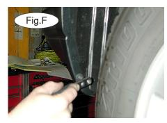
8. Remove the fascia by pulling forward from the edge of the fender well (Fig.I).
