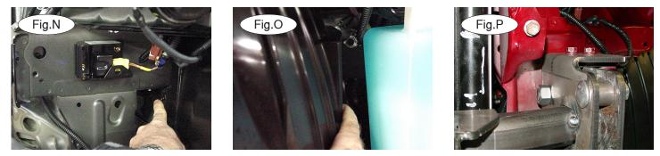
12. Working on the driver's side, put a  $\frac{1}{2}$ " x 2" carriage bolt through the rear mounting hole in a rear side mounting brace. Insert this brace into the front of the formed frame tube, with the rear bolt through a corresponding hole in the bottom of the frame. Secure with a  $\frac{1}{2}$ " nut, clipped plate washer, lock washer and nut (Fig.N). Leave loose at this time.
