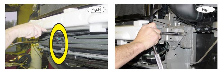
6. Remove the air temperature sensor and wiring harness from the bumper core by removing four plastic fasteners, if the vehicle is so equipped (Fig.H).
