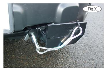
receiver braces are for padlocks only. Under no circumstances should you bolt the alignment tabs together. Bolting the alignment tabs together may result in non-warranty damage to the bracket.
