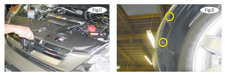
1. Important: please use all supplied bolts and parts and read all instructions carefully before beginning this installation. The majority of questions you may have can be answered within the text, and proper installation will ensure safe and secure travel. Now, begin the installation by removing seven plastic fasteners attaching the radiator cover to the core support (Fig.C).
