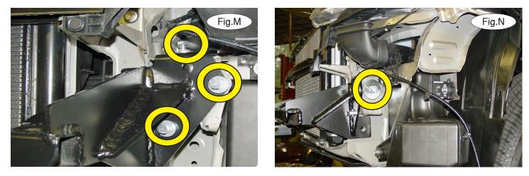
11. Working on one side at a time, use the supplied  $\frac{1}{2}$ " x  $1\frac{1}{2}$ " bolt, lock washer and plate washer and bolt through the main receiver brace and into the existing hole in the side of the frame rail (Fig.N). Repeat for the other side.
