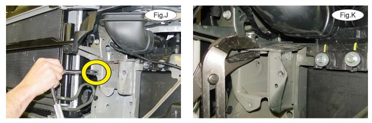
8. On each side, remove two 12mm (head) screws attaching the headlight support bracket to the end of the frame rail (Fig.J). *Note:* if there is a tab located on the top of the frame rail, it must be bent flush with the frame rail before installing the main receiver brace (Fig.K).
