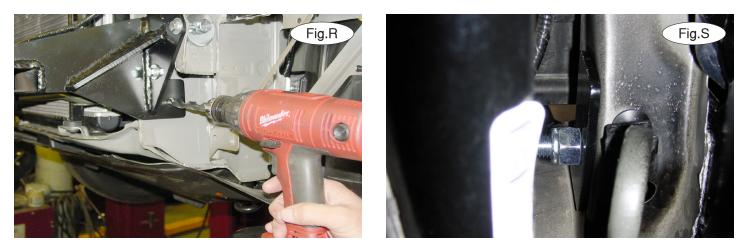
13. Remove the plastic fastener attaching the wiring harness to the inside of the core support on the driver's side. Now, on each side, using the pre-drilled hole in the main receiver brace as a template, drill through the existing hole in the outside of the core support and through the back side of the core support (Fig.R). *Note:* before drilling, make certain you will not drill into any engine components on the other side.
