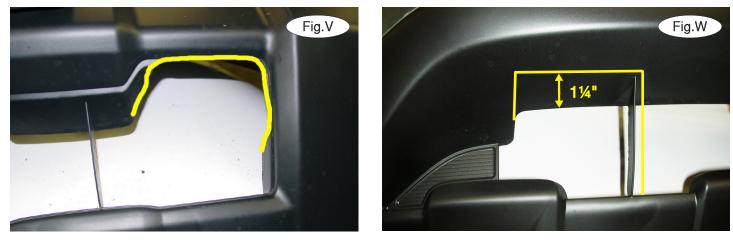
18. For '07 to '09 models: on each side, trim the fascia using the yellow lines in Figure V as a guide. For '10 to '11 models: on each side, measure up 1<sup>1</sup>/<sub>4</sub>" and trim straight over to the anchor of the vertical rib, using the yellow lines in Figure W as a guide for trimming.
