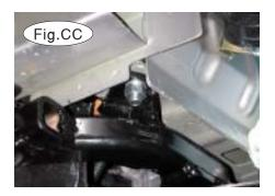
20. Then, fishwire one of the supplied  $\frac{1}{2}$ " x  $\frac{1}{2}$ " carriage bolts and  $\frac{1}{2}$ " x  $\frac{2}{2}$ " backing plates through the square opening in the frame rail (Fig.AA, Fig.BB) and through one of the holes you drilled in the preceding step. Thread a  $\frac{1}{2}$ " lock washer and nut over the bolt (Fig.CC), and torque the bolt to the specifications at the end of these instructions. Repeat for the other side.
