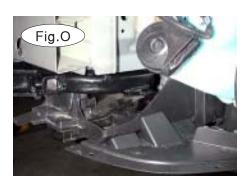
9. Trim both the driver's side and the passenger side air deflectors – Start by cutting away the sections marked with an 'X' in Figures M and N. Once the main receiver brace is bolted into place, trim the air deflectors to fit, as shown in Figure O.
