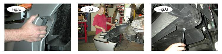
4. Pull out and away at each corner of the fascia (Fig.E). Then, remove the fascia (Fig.F).
