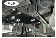
lock washers and nuts, to the passenger side of the side plate. Then, bolt the side plate to the main brace, using three 1/2" x 1<sup>1</sup>/<sub>2</sub>" bolts, lock washers and nuts (each side).
