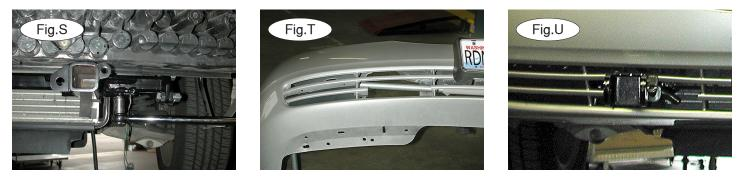
13. Tighten the bolts. Start with the lower bolt that passes through the frame rail (Fig.S). Then, tighten the bolts on the upper core support. This pulls the bracket up and into place. Then, tighten the remaining side plate bolts (five on each side).
