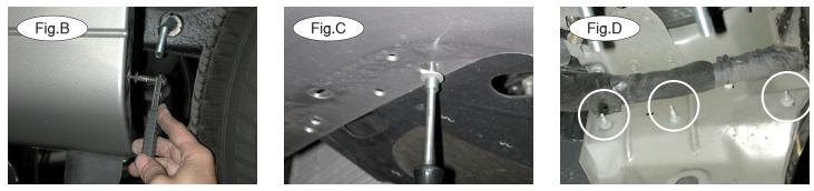
1. *Important:* please use all supplied bolts and parts and read all instructions carefully before beginning this installation. The majority of questions you may have can be answered within the text, and proper installation will ensure safe and secure travel. Now, begin the installation. Start by removing one Phillips head screw on the edge of the fender well, on each side (Fig.B).
