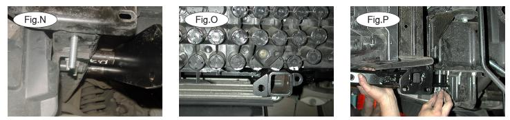
9. Now, reinstall the bumper core by reversing step 6. Trim the plastic bumper absorption plate by cutting eight inches in from the outside, and level with the bottom of the bumper core. (Refer to the white line in Fig.O.)
