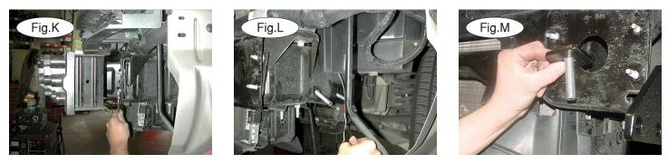
6. Remove the four 13mm nuts on each side of the bumper core (Fig.K). Then, remove the bumper core.
