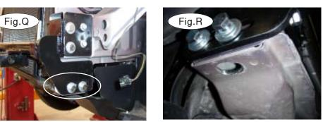
6. Using the lower mounting points in the main receiver brace, bolt the main receiver brace to the radiator support using the two 10mm x 1.5 x 35mm bolts, fender washers and lock washers (Fig.Q). *Note:* due to manufacturing variances, some vehicles may not be equipped with factory weld nuts. Enlarge the hole in the bottom of the frame and then use the four supplied 10mm fender washers, lock washers and nuts instead of the weld nuts (Fig.R).
