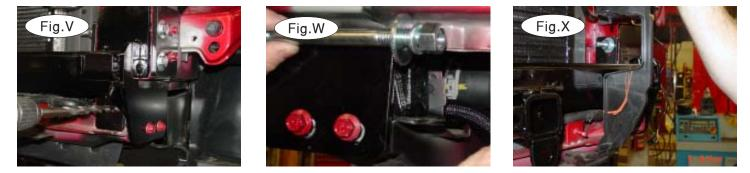
8. Using the main receiver brace as a drill template, drill a 17/32" hole through the front of the frame on each side (Fig.V).
