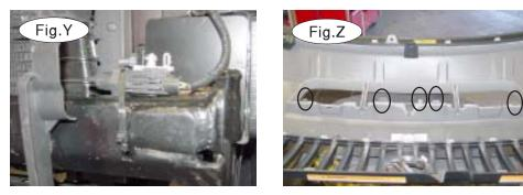
12. If the vehicle is equipped with an ambient temperature sensor, reattach it to the main receiver brace using the two provided zip ties (Fig.Y).
