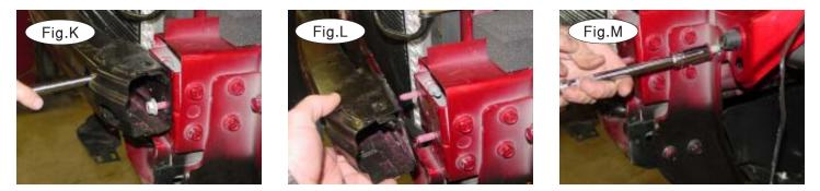
4. Now remove the tie down brackets (five 13mm head bolts) on each side (Fig.M), then remove the bumper core support brackets in front of the frame tubes (four 13mm head bolts) on each side (Fig.N).
