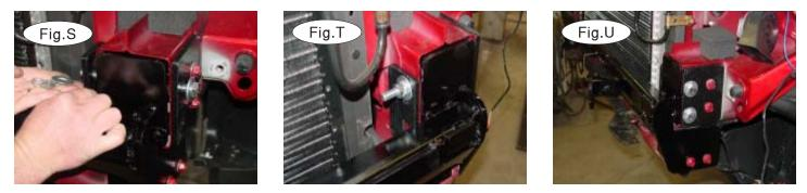
7. Bolt through the top front frame mounting holes, the outside backing plate and an inner backing plate with two 10mm x 1.5 x 140mm bolts, fender washers, lock washers and nuts on each side (Fig.S,T,U).
