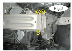
Next, remove the bumper core. *Note*: the bumper core will not be re-installed.
