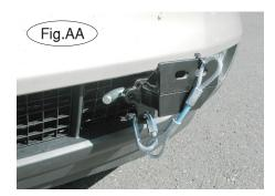
22. Install the tow bar to the mounting bracket according to the manufacturer's instructions.
