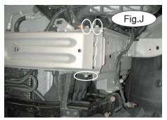
Note: retain the bumper core and attachment hardware so that it can be replaced if the bracket is ever removed.
