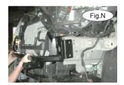
14. Next, reattach the core support to the main receiver brace using the 10mm (head) bolts you removed in step 8 on the upper holes only (Fig.P) and use the supplied 8mm x 1.25 x 35mm bolt, 8mm lock washer and 5/16 flat washer on the lower hole. *Note:* use thread lock on the factory bolts prior to reinstalling them. **Make certain that the power steering cooler lines are not contacting the**
