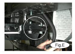
3. Hold the receiver brace and shim plate for that side flat against the tow loop mounting plate and the bottom of the frame (Fig.D). Bolt in place with two of the supplied 12mm x 60mm bolts, flat washers and lock washers (Fig.E) *Note:* compare the thread of the supplied bolts to the original bolts. We have found both 1.5 and 1.75 thread pitch bolts in these vehicles. Bolts with both thread pitches are supplied in the kit.
