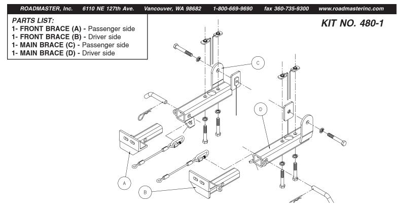
**IMPORTANT:** All baseplates **must** be assembled with all the bolts left loose for final adjustment and positioning (before tightening) unless otherwise instructed. All bolts **must** be torqued for proper strength. If more than one bolt is used per fastening point, the diagram may only show one. Use flat washers over all slotted holes and lock washers on all fasteners.
