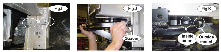
6. Next, remove four 12mm head bolts attaching the bumper core to the frame rail, two per side (Fig.I)
