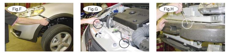
4. Now, pull out and forward on both corners of the fascia (Fig.F). Then, pull up on the lock tabs holding the top of the fascia to the core support to remove the fascia (Fig.G).
