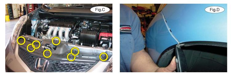
1. *Important:* please use all supplied bolts and parts and read all instructions carefully before beginning this installation. The majority of questions you may have can be answered within the text, and proper installation will ensure safe and secure travel. Now, begin the installation. Remove five plastic fasteners attaching the top of the fascia to the core support (Fig.C).
