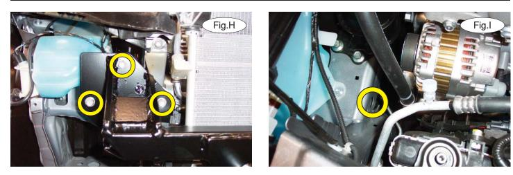
6. Place the main receiver brace over the ends of the frame rails. On each side, replace the four bolts removed in the previous step. *Note:* Figure H only shows three bolts. The fourth is below the brace.
