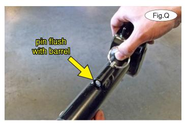
The spring-loaded pin on the removable arm snaps into a notch on the receiver, locking the removable arm into its final towing position. Before inserting each arm into the receiver, verify that the spring is working by ensuring that the spring-loaded pin moves easily back and forth within the barrel when pulled and that it can be pulled flush with the face of the barrel (Fig.P and Fig.Q).
