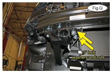
15. On each side, finish the two  $\frac{1}{2}$ " x 1<sup>1</sup>/<sub>4</sub>" bolts on the inside holes of the spacer plate and main receiver brace by adding two  $\frac{1}{2}$ " lock washers and nuts (Fig.Q).
