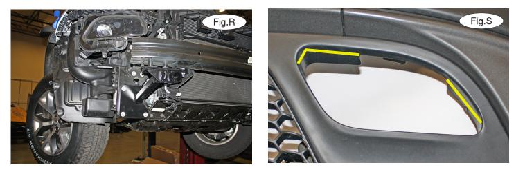
16. On each side, replace the three 15mm (head) bolts you removed in step 10 (Fig.R).
