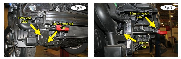
11. On each side, use a cut-off wheel to remove the exposed stud and use a hammer to flatten the alignment tab (Fig.M). 12. On each side, remove two 16mm (head) bolts attaching the tow hooks to the bottom of the bumper core. Now, use a crescent wrench on the 30mm nut attaching the tow hook to the rear of the tow hook bracket and then twist the front of the tow hook back and forth by hand to aid in removing the nut (Fig.N).
