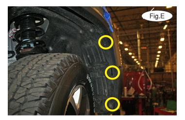
3. On each side, remove three 8mm (head) screws attaching the fender liner to the fascia (Fig.E).
