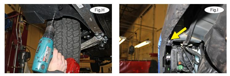
6. On each side, use a ¼" drill bit to remove the plastic pop rivet attaching the bottom of the fascia to the fender liner (Fig.H).
