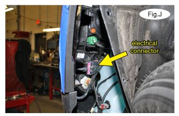
8. On the driver's side only, disconnect the purple electrical connector and a plastic fastener attaching the wiring loom to the core support (Fig.J). *Note:* make certain that the vehicle is not turned on while this connector is unplugged or it may trigger the 'Check Engine' light to illuminate.
