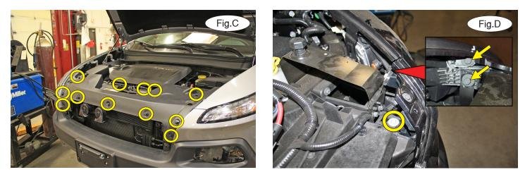
1. *Important:* please use all supplied bolts and parts and read all instructions carefully before beginning this installation. The majority of questions you may have can be answered within the text, and proper installation will ensure safe and secure travel. Now, begin the installation by removing 12 plastic fasteners attaching the radiator cover to the core support (Fig.C).
