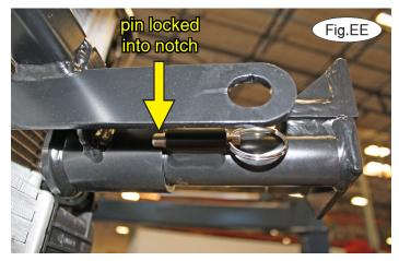
24. On each side, insert the removable front bracket arm into the front receiver 90 degrees from its final towing position, depressing the spring-loaded pin against the receiver (Fig.DD). Now, twist back 90 degrees until the spring-loaded pin snaps into place in the notch on the receiver, locking the arm into place in its final towing position (Fig.EE).
