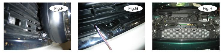
4. If the vehicle is equipped with fog lights, remove two 4mm Allen head screws on each side (Fig.F), and pull forward to release each light from the fog light mount (Fig.G). Now, remove four plastic fasteners attaching the top of the grille to the core support (Fig.H).
