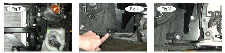
16. Position the main receiver brace over the ends of the frame rails so that the three pre-drilled holes at each end of the main receiver brace align to the holes for the 13mm (head) nuts you removed in step 12 (Fig.T). Reattach the 13mm (head) nuts, through the main receiver brace and into the ends of the frame rails.
