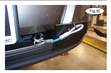
*Note:* if the bracket is so equipped, the holes in the alignment tabs which are welded to the arms and main receiver braces are for padlocks only. Under no circumstances should you bolt the alignment tabs together. Bolting the alignment tabs together may result in non-warranty damage to the bracket.
