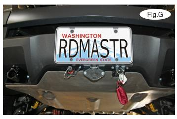
5. On each side, remove two 15mm (head) bolts attaching the front skid plate to the frame. Then, loosen the two rear 15mm (head) bolts attaching the front plate to the rear skid plate to remove it (Fig.F). *Note:* if you plan to use a breakaway and/or our wiring plug mounts, you will need to trim the skid plate as shown in Figure G.
