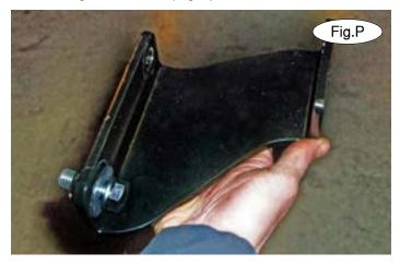
13. On each side, insert one of the supplied 3/16" x  $1\frac{1}{2}$ " x 3" threaded backing plates without rod into the bottom of the subframe (Fig.O). Arrange the hardware for the rear support plate for each side as shown in Figure P, with the  $\frac{1}{2}$ " x 2" bolt,  $\frac{1}{2}$ " lock washer,  $\frac{1}{2}$ " flat washer, and finish with the 1" O.D. x  $\frac{1}{4}$ " x .188 wall pipe spacer and loosely bolt into the threaded backing plate in the bottom hole of the subframe.
