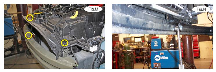
10. On each side, remove two 10mm (head) bolts attaching the core support to the bumper core and one 10mm (head) bolt attaching the hood latch support to the bumper core (Fig.M).
