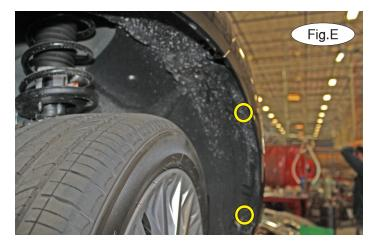
3. On each side, remove two T25 Torx bolts attaching the fender liner to the fascia (Fig.E).
