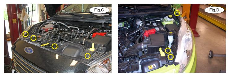
1. *Important:* please use all supplied bolts and parts and read all instructions carefully before beginning this installation. The majority of questions you may have can be answered within the text, and proper installation will ensure safe and secure travel. Now, begin the installation. Remove four plastic fasteners attaching the radiator cover to the core support (Fig.C).
