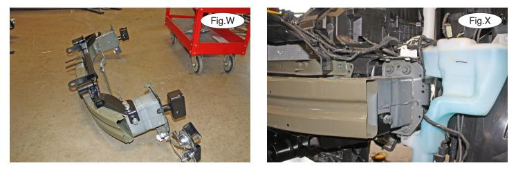
20. Repeat steps 16 through 19 for the driver's side. Figure W shows the bumper core with the main receiver brace fully installed.
