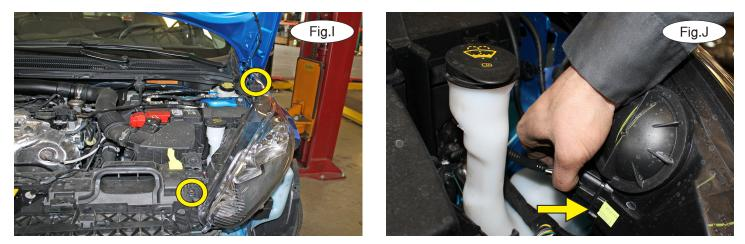
6. On each side, remove two T30 screws attaching the headlight to the frame (Fig.I). Then, unplug the wiring harness (Fig.J) and carefully lift the headlight out and set it aside.
