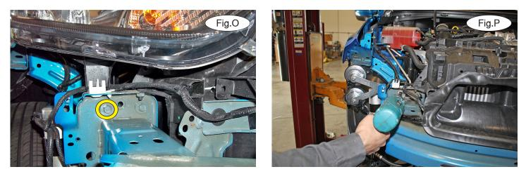
9. On each side, remove the upper- and outermost 13mm (head) bolt attaching the bumper core to the frame rail (Fig.O). Now, using a 9/16" drill, drill out the remaining weld nut (Fig.P).
