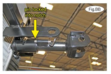
22. On each side, insert the removable front bracket arm into the front receiver 90 degrees from its final towing position, depressing the spring-loaded pin against the receiver (Fig.AA). Now, twist back 90 degrees until the spring-loaded pin snaps into place in the notch on the receiver, locking the arm into place in its final towing position (Fig.BB).
