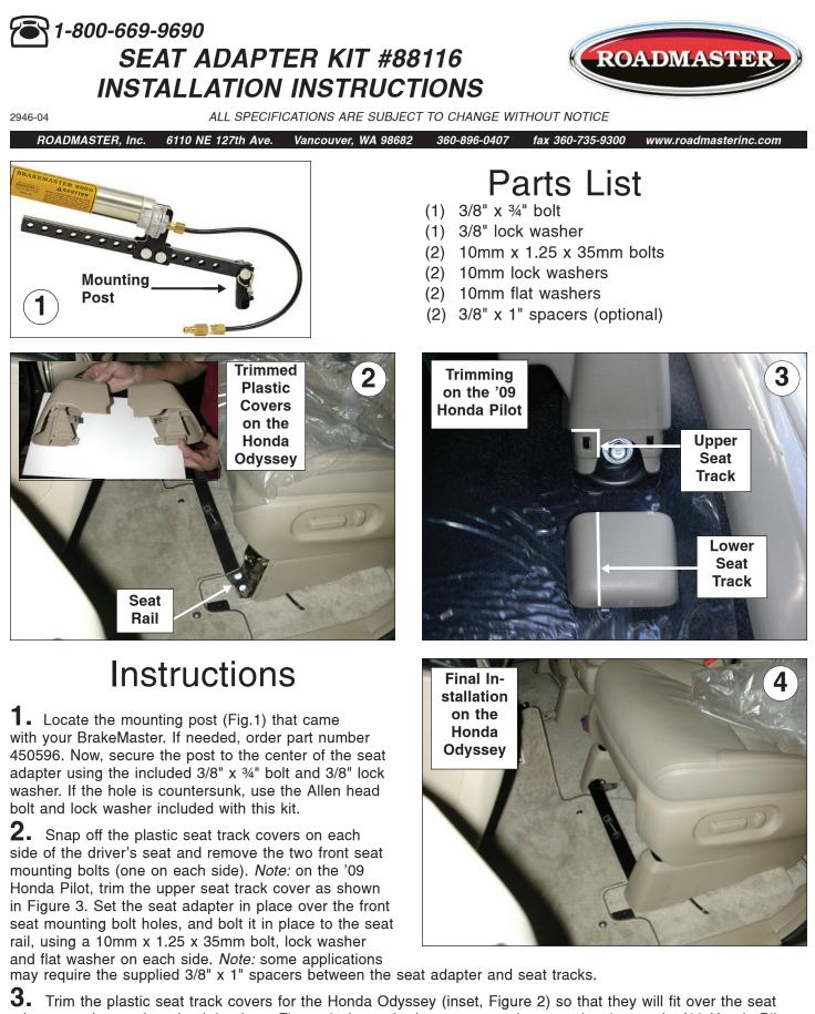
adapter, and snap them back in place. Figure 3 shows the lower seat track cover trimming on the '09 Honda Pilot.
