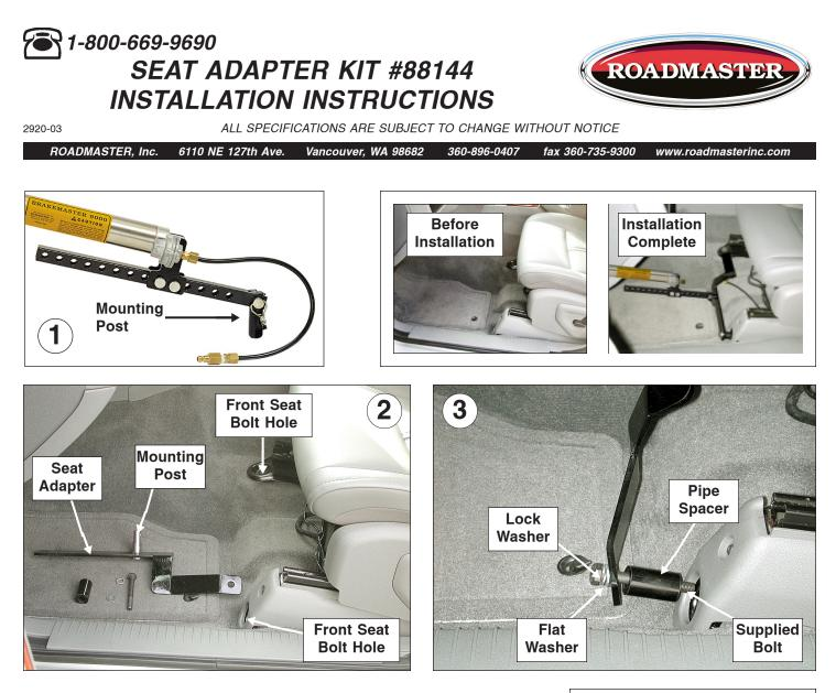
**1.** Locate the mounting post (Fig.1) that came with your BrakeMaster. If needed, order part number 450596. Now, secure the post to the center of the seat adapter using the included  $3/8^{\circ} \times 3/4^{\circ}$  bolt and  $3/8^{\circ}$  lock washer. If the hole is countersunk, use the Allen head bolt and lock washer included with this kit.
