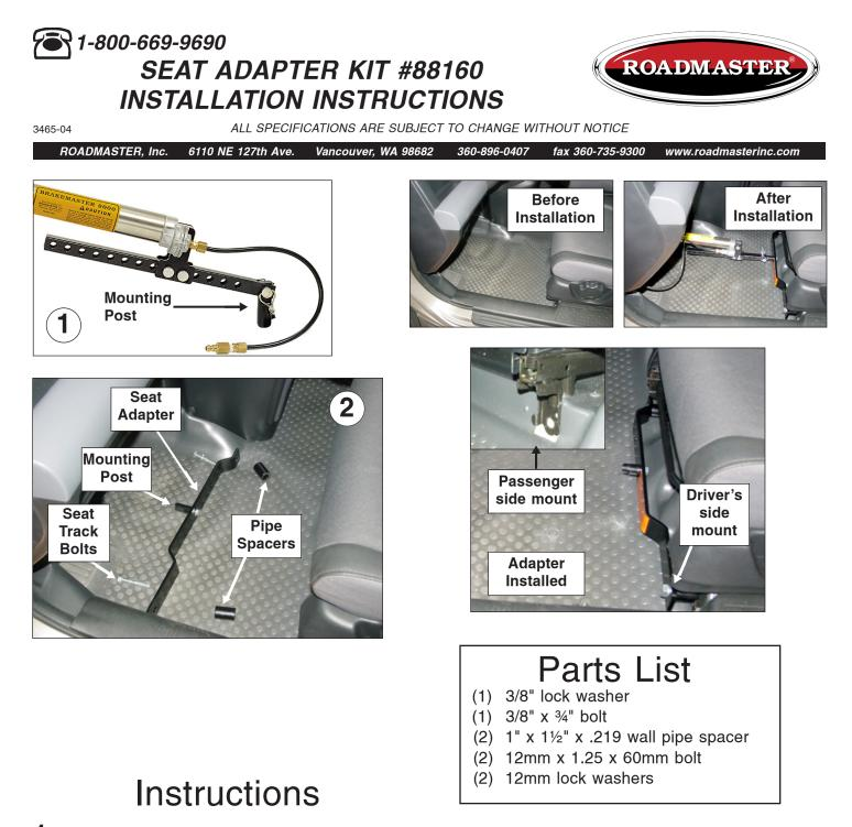
**1.** Locate the mounting post (Fig.1) that came with your BrakeMaster. If needed, order part number 450596. Now, secure the post to the center of the seat adapter using the included 3/8" x <sup>3</sup>/<sub>4</sub>" bolt and 3/8" lock washer. If the hole is countersunk, use the Allen head bolt and lock washer included with this kit.
