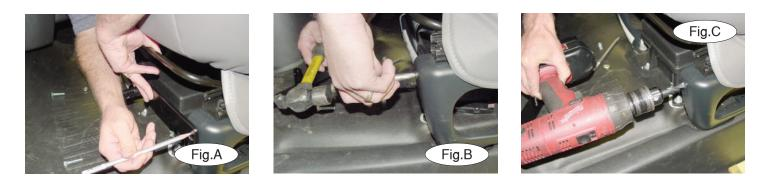
**2.** Hold the bracket in place over the end of the seat pedestal. Using the two existing holes in the adapter as a template mark each side for drilling (Fig.A). Center punch the areas you marked (Fig.B), then, drill the two holes using a 3/8" drill (Fig.C). Now, put the seat adapter over the holes you drilled and bolt into place using the supplied 3/8" x 1<sup>1</sup>/<sub>4</sub>" bolts, lock washers and nuts (Fig.D).
