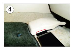
**5.** Replace the seat track covers and trim to allow clearance for the seat adapter using the red lines in Figure 4 as a guide for trimming.
