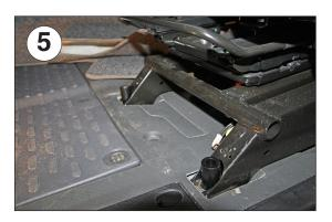
**4.** Place the supplied 1" O.D. x .188 wall pipe spacers over the holes you just exposed in the previous step (Fig.5).
