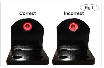
2. Install the tie rod bracket to the barrel end of the steering stabilizer with the long side of the bracket pointing toward the passenger side of the vehicle. *Note: Ensure the bushings are oriented in the tie rod bracket hole as shown in Figure 1. Proper orientation of the bushing will keep the Reflex unit centered in the bracket. Note that the bracket shown in Figure 1 may vary by kit.*
