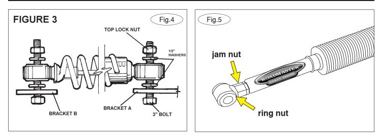
4. Place one three-inch bolt through the top side of the chassis bracket through the 1/2" bolt hole (Fig.4). Place one of the provided 1/2" flat washers and the stabilizer loop mount over the bolt. Place another 1/2" flat washer over the bolt to rest on the loop mount, and one of the provided 1/2" lock nuts over the bolt. Finger-tighten only at this time.
