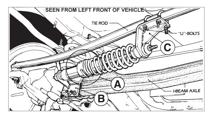
Note: Before installing the shock component of this system, please ensure that the spring is fully-seated in its track on the collar of the unit. If it is installed without the spring fully-seated in its track, the unit could malfunction or otherwise fail to operate properly (A).
