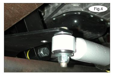
4. Place one three-inch bolt through the top side of the chassis bracket through the 1/2" bolt hole. Place one of the provided 1/2" flat washers and the stabilizer loop mount over the end of the bolt. Place another 1/2" flat washer over the bolt to rest on the loop mount, and one of the provided 1/2" lock nuts over the bolt. Finger-tighten only at this time (Fig.4).
