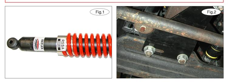
Note: Roadmaster makes multiple steering stabilizers. The unit depicted in these instructions may vary from your unit but all stabilizers will follow these instructions. If installing a Reflex, ensure that the spring is fully-seated in its track on the collar of the unit. If it is installed without the spring fully-seated in its track, the unit could malfunction or otherwise fail to operate properly (Fig.1).
