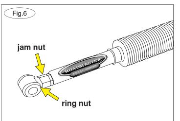
unit in place so that it does not rotate when you tighten the jam nuts. Test drive the vehicle and ensure that it is not pulling to the left or right. If it needs to be adjusted, follow step 8. Note: Due to manufacturing variances, the decals may be situated on either the passenger side or the driver's side of the vehicle. This does not impact the product's functionality or how it is installed, as the unit is bi-directional.
