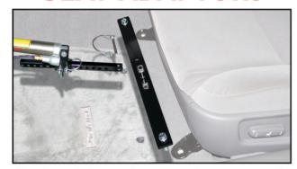
Provide a vehicle-specific mounting location to pin the BrakeMaster. Available for most vehicles; required on some applications.
