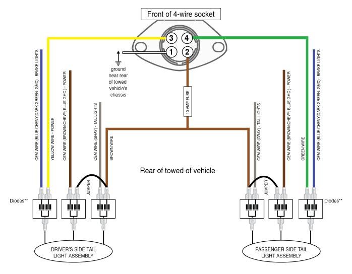
To power up the tail light assemblies on the Chevy Silverado 2500/3500 or GMC Sierra 2500/3500, simply plug in the dinghy to the motorhome and turn ON the headlights on the motorhome.
