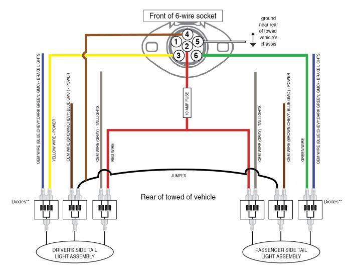
To power up the tail light assemblies on the Chevy Silverado 2500/3500 or GMC Sierra 2500/3500, simply plug in the dinghy to the motorhome. The 12V charging circuit will always have power.
